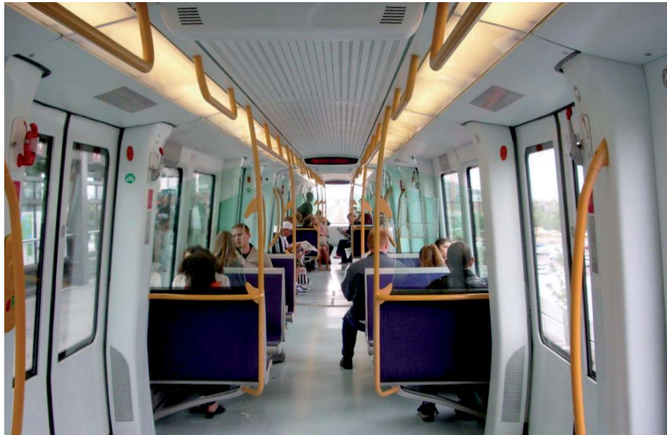
Fig. 23: The seats of the metro in Copenhagen are suspended from the wall. Thus, dogs and baggage find space under the seat and cleaning is easier.
